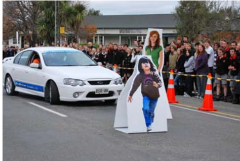
At 50kph without ABS, the rear of the car starts to slide
