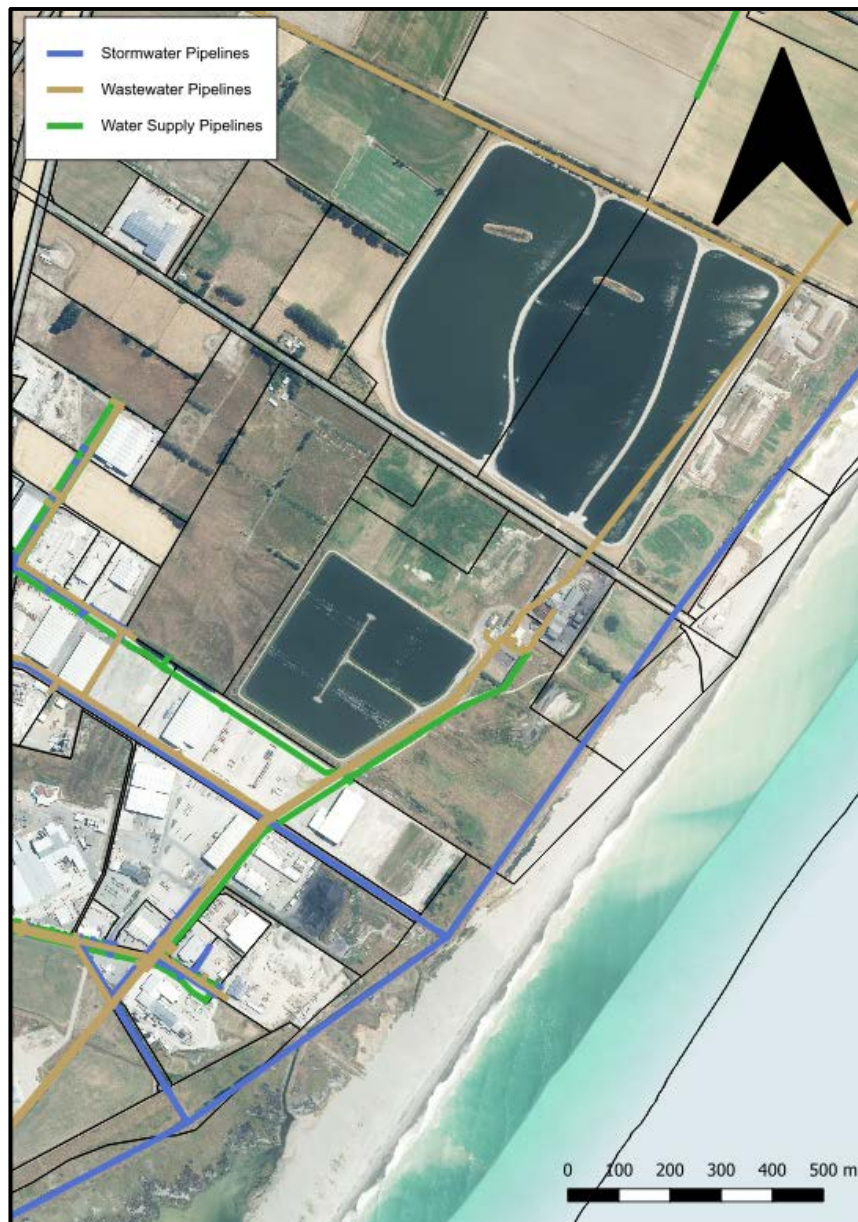
Figure 11: Stormwater, wastewater, and water supply pipelines within the site of interest.
