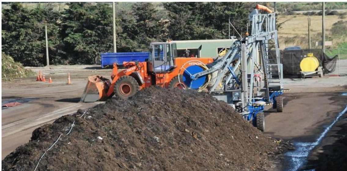
Compost is turned from one windrow to another three times in the eight week processing cycle, providing aeration and mixing the materials.
