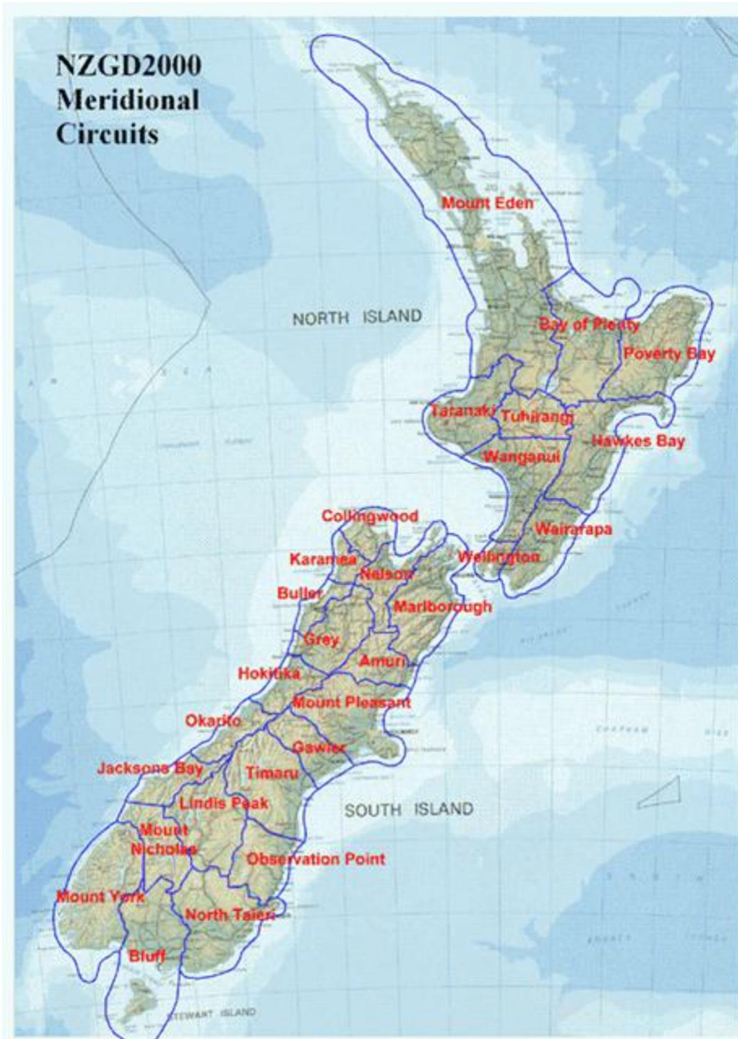
Figure 1 NZGD2000 Meridional Circuits
