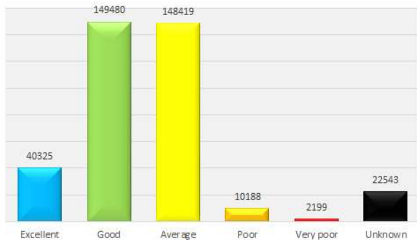
Fig 82: Kerb and channel condition ratings
