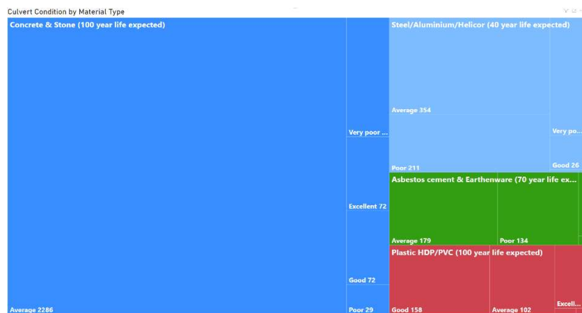
Fig. 79: Culvert condition by material type. This shows the breakdown of culvert material types linked to assumed condition and expected life. Not all culvert materials will have a uniform expected life due to the different deterioration cycles of each material used. Average condition metal pipes steel and aluminium will need replacing a lot faster than concrete or PVC culverts due to the reduced life expected due to material oxidation in saturated environments.
