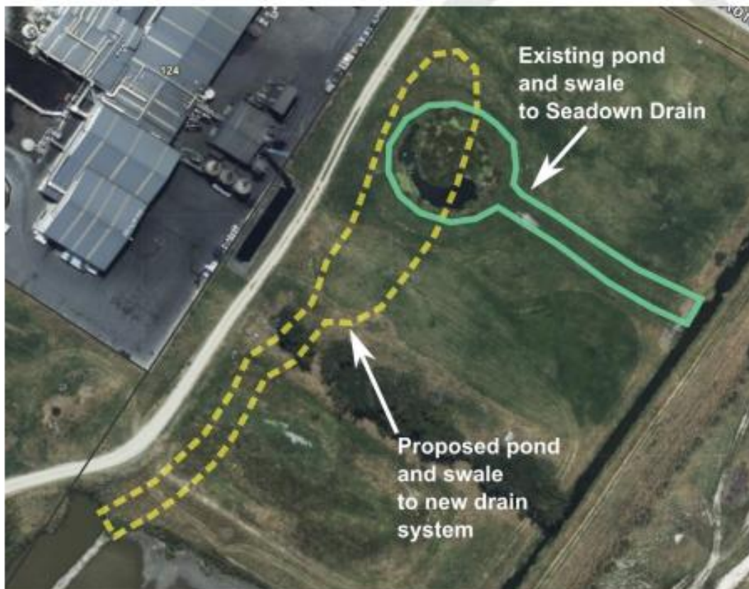
Figure 11: Schematic of FBNZ retention basin replacement
