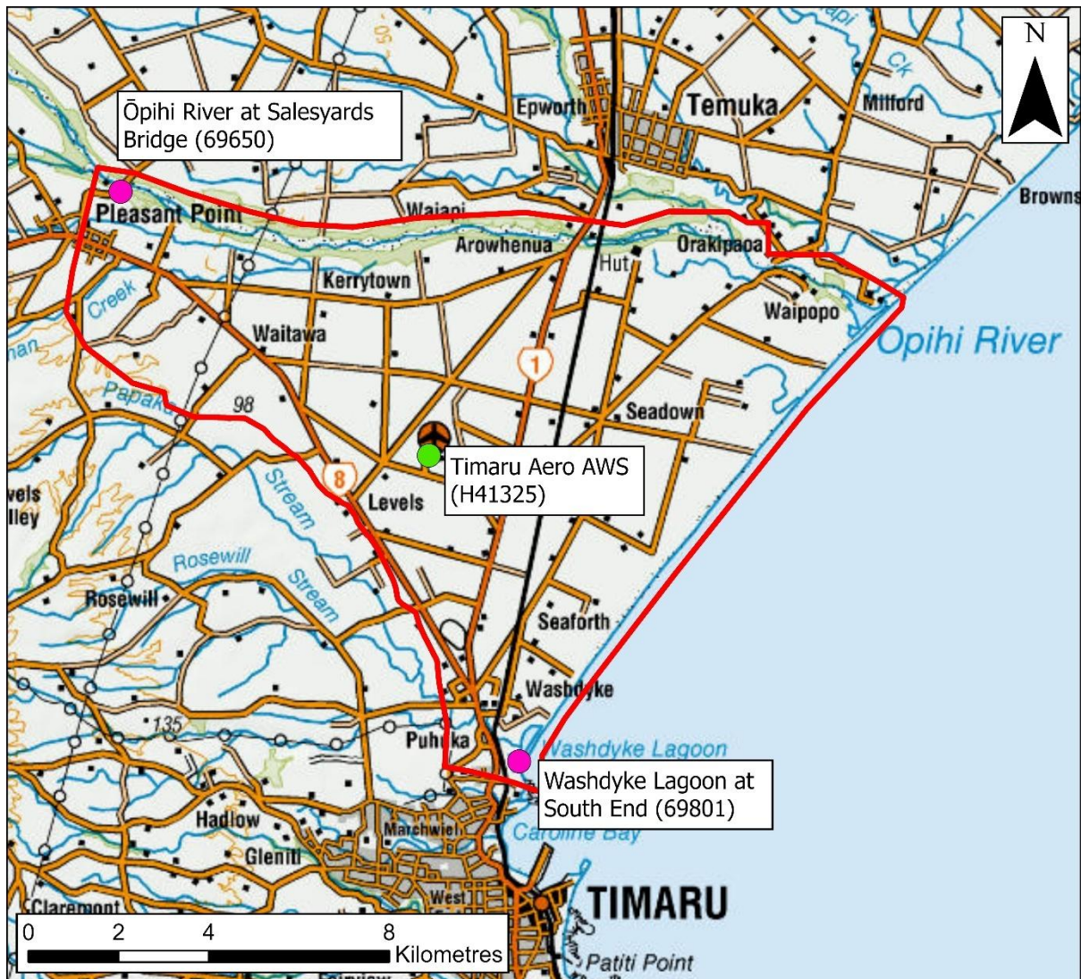
Figure 2: Model study area (red outline) and location of water level and flow gauges (pink) and rainfall recorders (green) used for modelling
