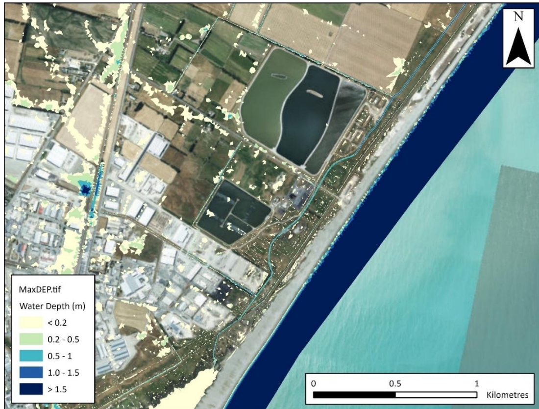
Figure 22: Maximum modelled water depth – proposed stopbank configuration with Rifle Range – mean annual rainfall – Zoomed to Washdyke area
