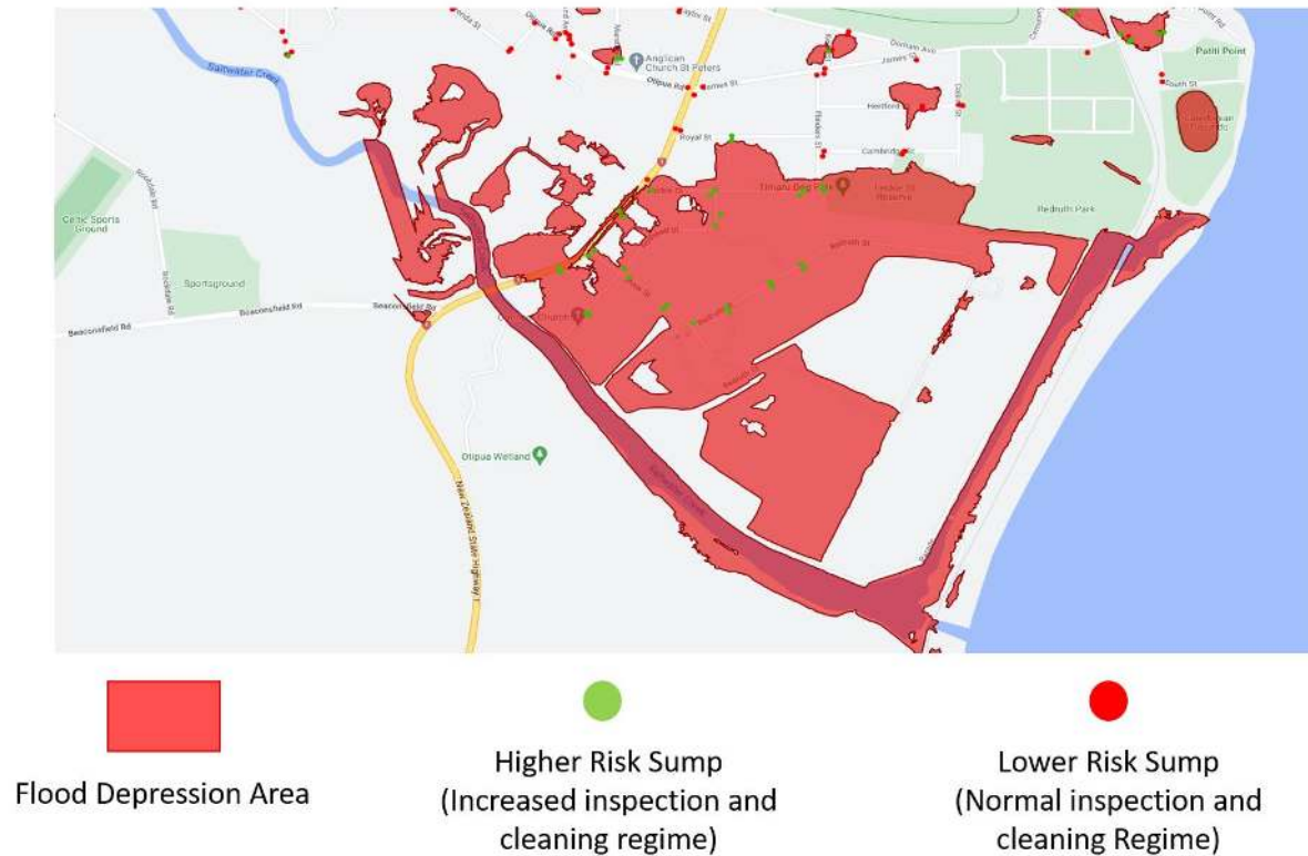
Fig 84: This is an overlay of identified flood depression areas with sump data to help identify sumps and culverts that are located in low lying areas of the district. Using this data, sump inspection and cleaning frequencies in these areas is done on a more regular basis, and during periods of high rainfall cyclic patrols undertake additional inspections to ensure that the sumps are not blocked and working to the full capacity of their design.
