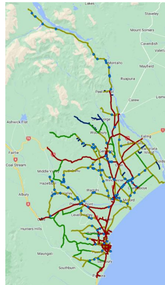
Fig. 57: Critical assets are mapped in RAMM, indicating what part so of the network are Critical , High , Medium or Low priority
