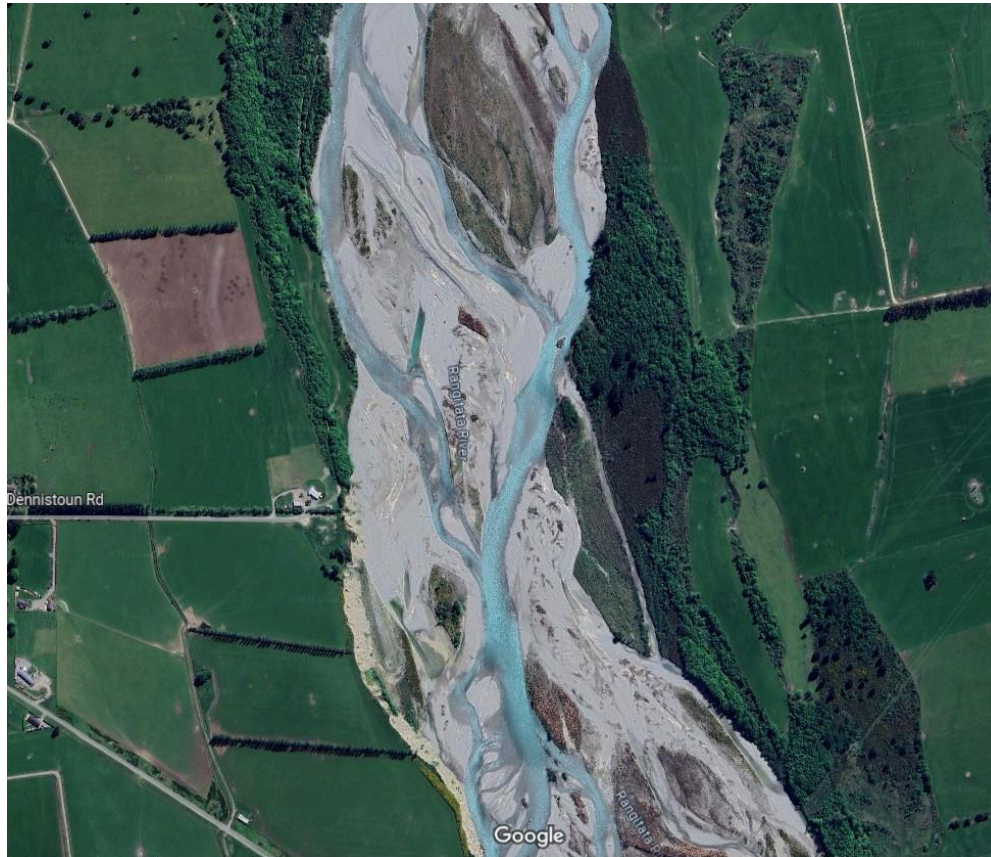
Aerial photograph showing channel alignment changes and in-river guide banks (google maps).
