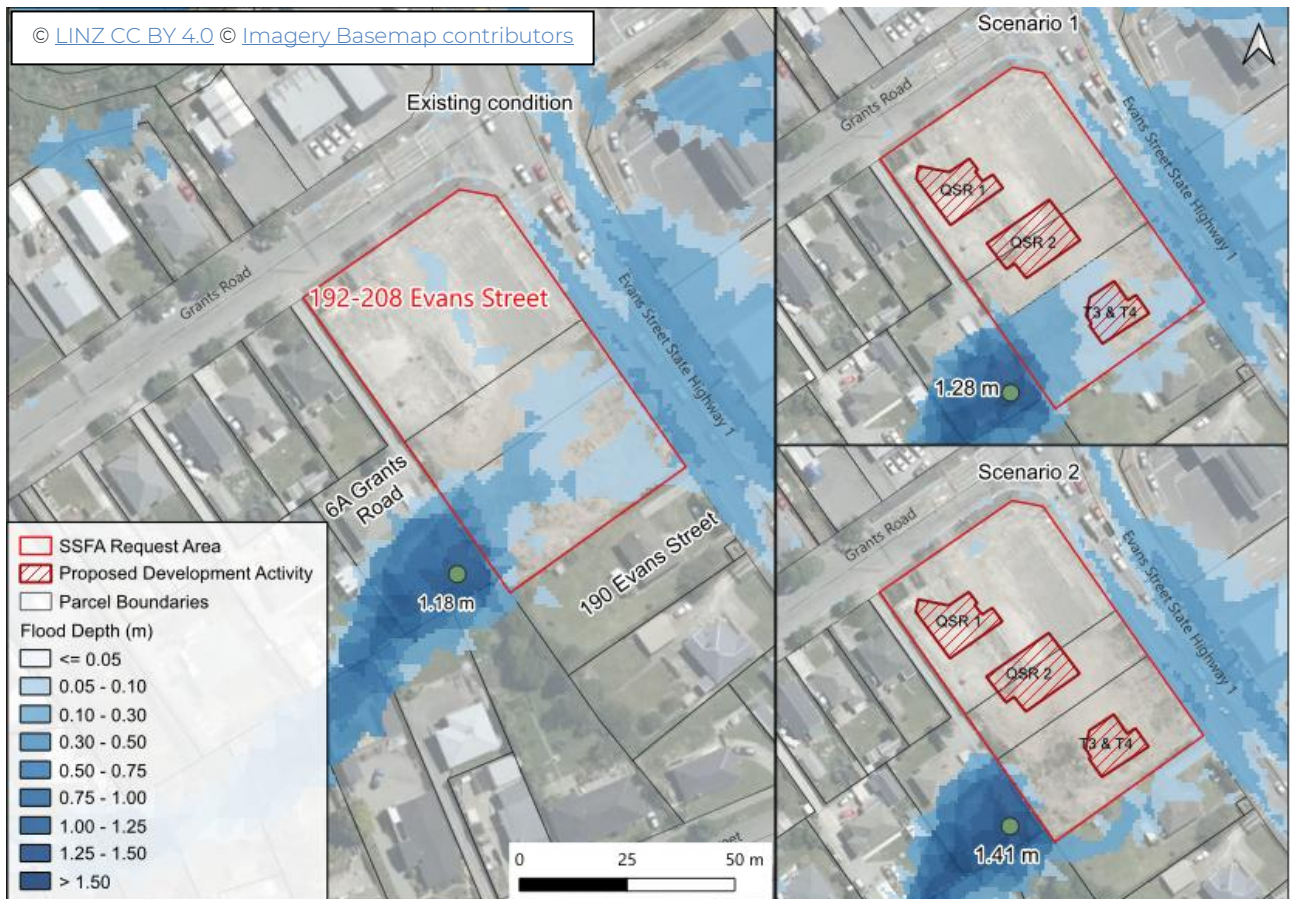
Figure 2-10: Modelled water depths [m] during the 10% AEP rainfall event (without climate change), comparing existing condition with Scenario 1 and Scenario 2 .
