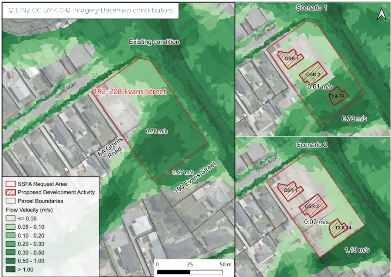
Figure 2-12: Modelled flow velocities [m/s] during the 0.5% AEP rainfall event (includes an allowance for climate change).
