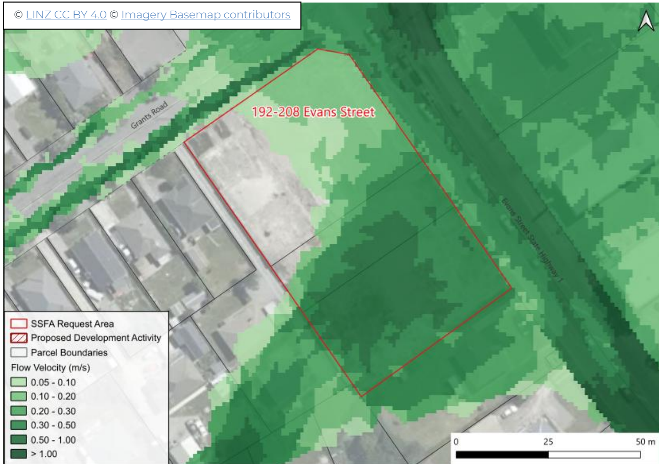
Figure 2-11: Modelled flow velocities [m/s] during the 0.5% AEP rainfall event (includes an allowance for climate change). Existing site ground surface created from LINZ – Canterbury LiDAR 1m DEM (2020-2025).
