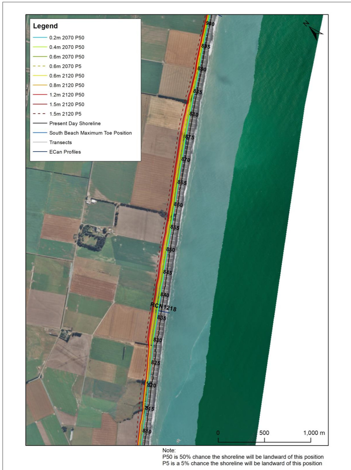
Figure 5.17: Orari River to the Rangitata River (north) PFSP for various SLR scenarios in 2070 and 2120. 'Most likely' position (P50) is shown for each scenario, and 'very unlikely' (P5) is shown for SLR scenarios of 0.6 m by 2070 and 1.5 m by 2120 (highest SLR scenario).
