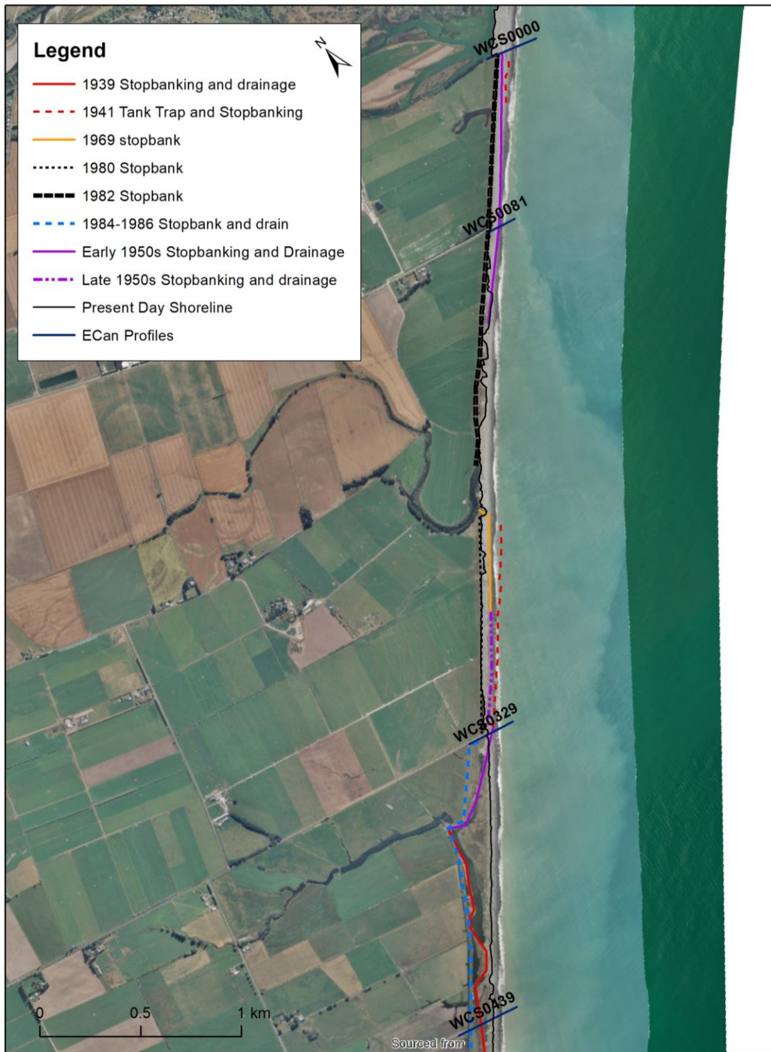
Figure 5.8: Northern Seadown coastal stopbank locations
