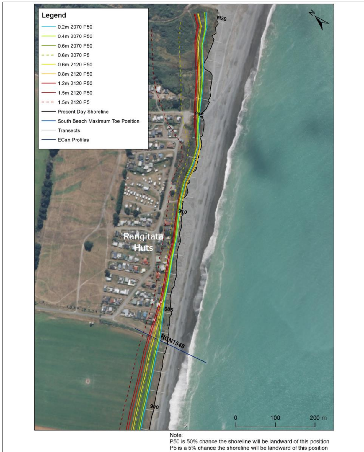
Figure 5.19: Rangitata Huts PFSP for various SLR scenarios in 2070 and 2120. 'Most likely' position (P50) is shown for each scenario, and 'very unlikely' (P5) shown for SLR scenarios of 0.6m by 2070 and 1.5m by 2120 (highest SLR scenarios).
