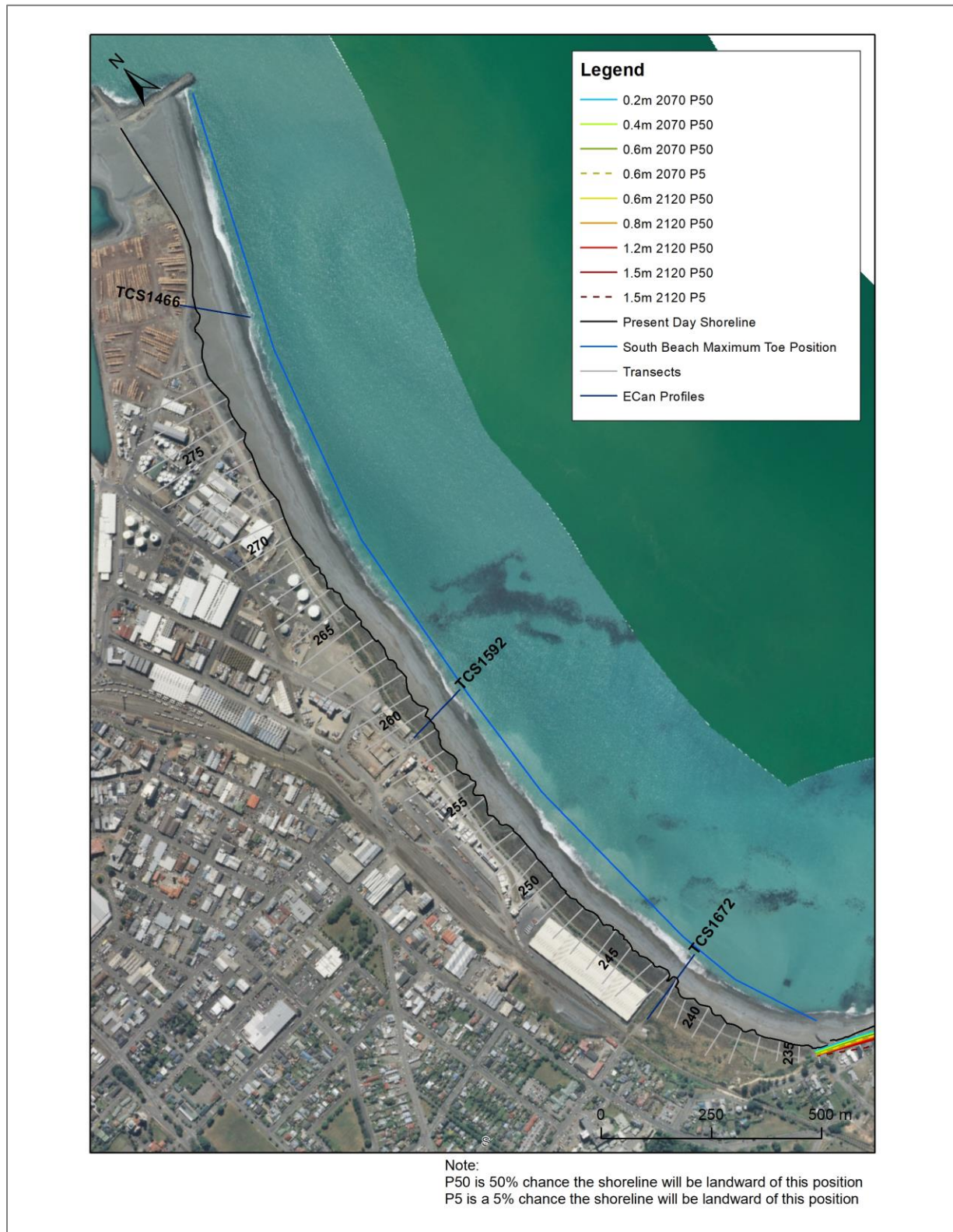
Figure 4.5: Projected maximum South Beach toe position.
