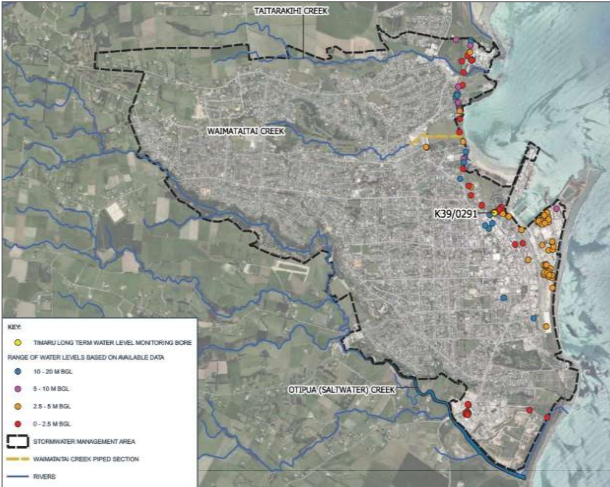
Figure 5-10 Depth to groundwater
