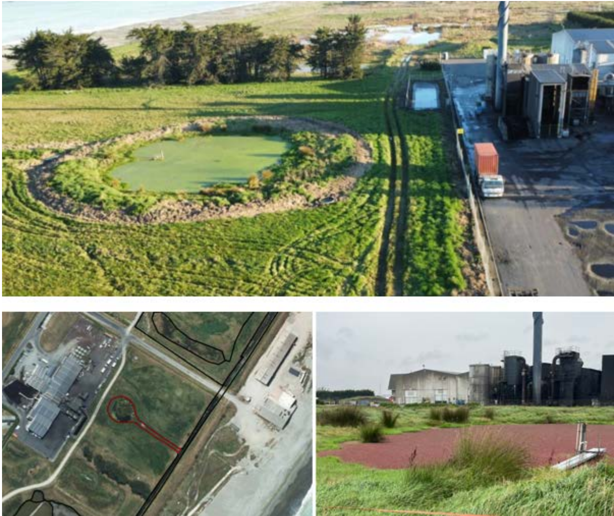
Figure 5 The existing extent of the ‘retention pond’ wetland south of Aorangi Road. This waterbody, considered an ‘RMA wetland’ rather than a ‘natural inland wetland’, was created for stormwater retention (not treatment) purposes.
