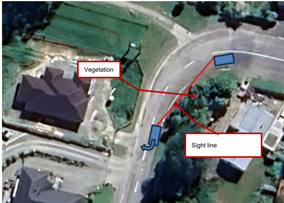
Figure 1 – sight line to a vehicle turning right into 2 Gresham Street
