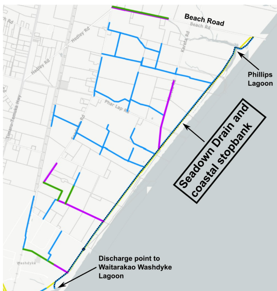
Figure 1: Schematic of Seadown drainage system. The Seadown Drain/coastal stopbank is dotted, other drains are shown as blue, purple and green lines, yellow lines are stopbanks. (Base image source: Canterbury Maps)
