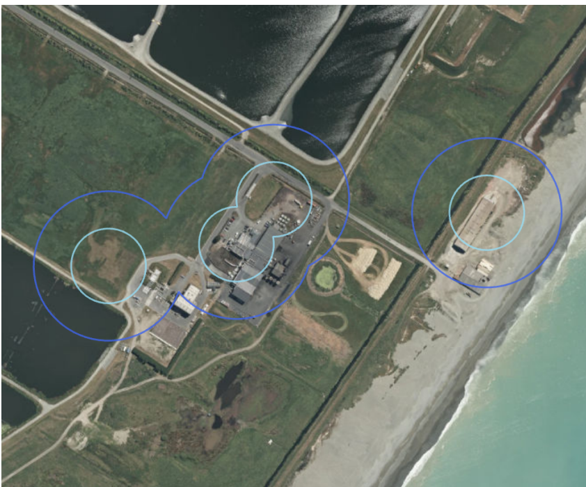
Figure 19: PTDP drinking water protection areas; pale blue circle is 50 m buffer from bore, dark blue 100 m (Source: TDC planning maps).
