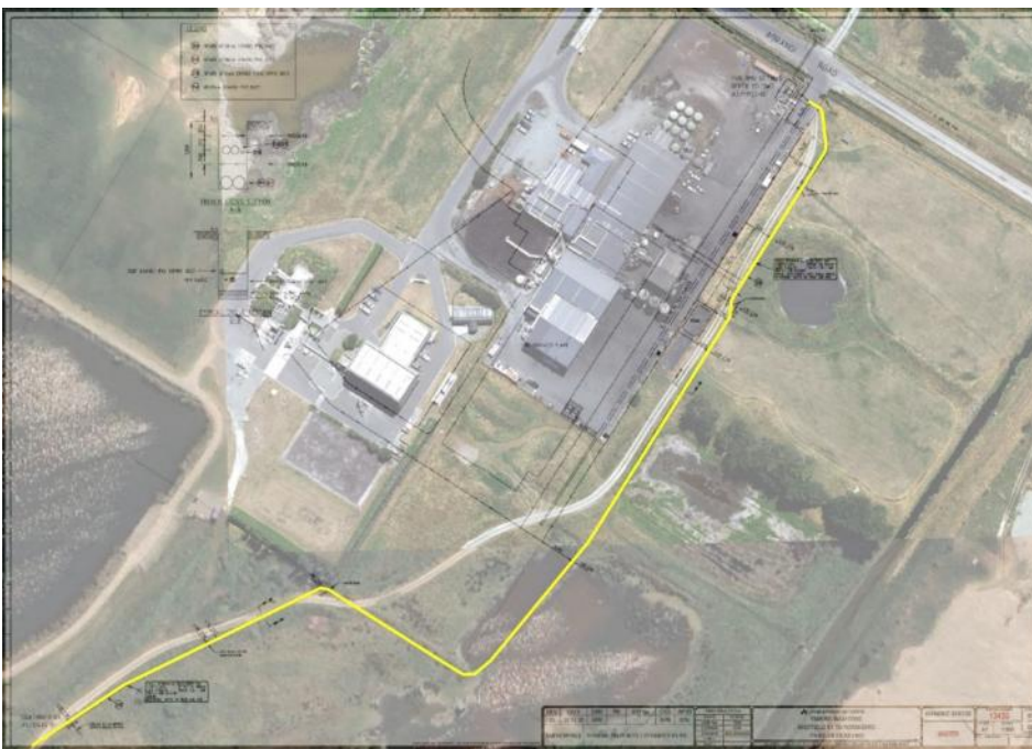
Figure 14: Alpine Energy 11kV cable location (yellow line).
