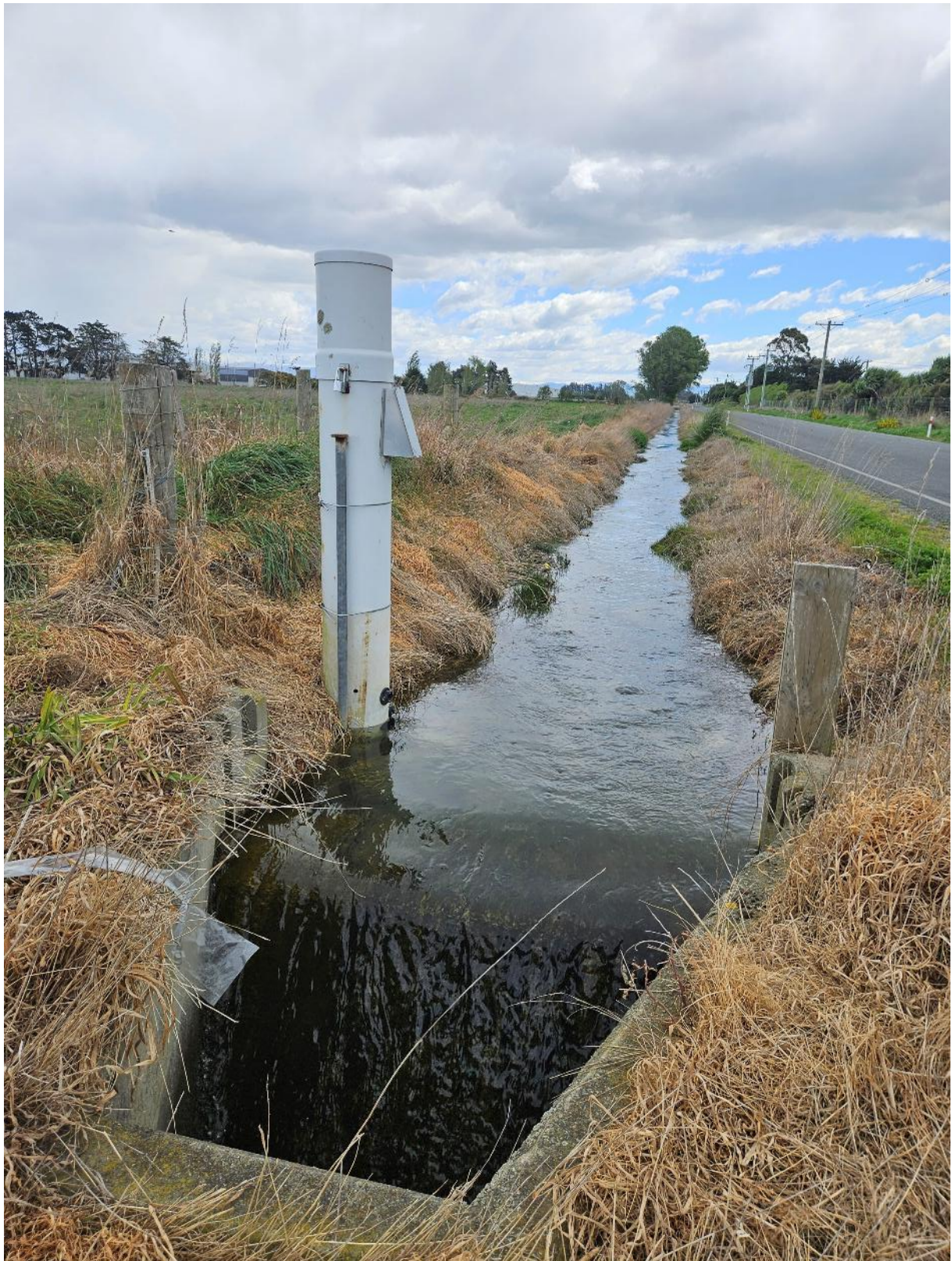
Figure I16: Stage Gauge and Weir at Aorangi Road (Connecting to Seadown Main Drain)
