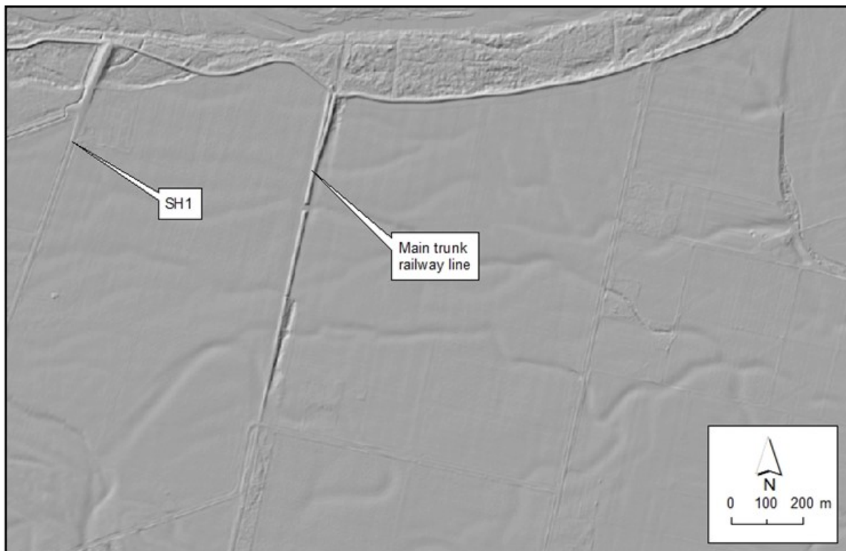
Figure A1-3: Comparison of aerial imagery and LiDAR (ground level) data (1m DEM)
