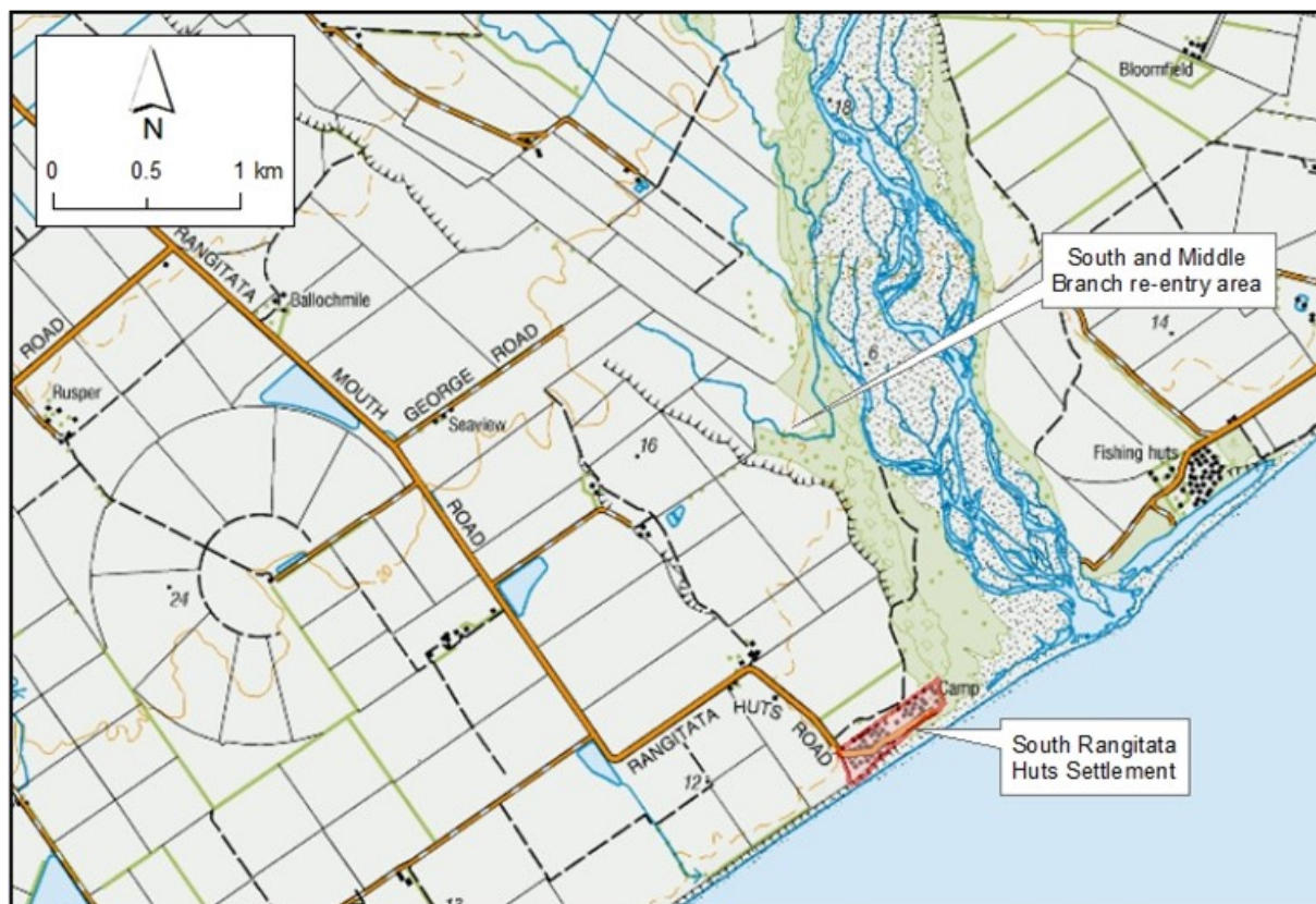
Figure 2-7: Location where South and Middle Branches of the Rangitata River re-enter the main river channel. The natural terrace downstream of this point has historically prevented floodwater continuing down toward the huts
