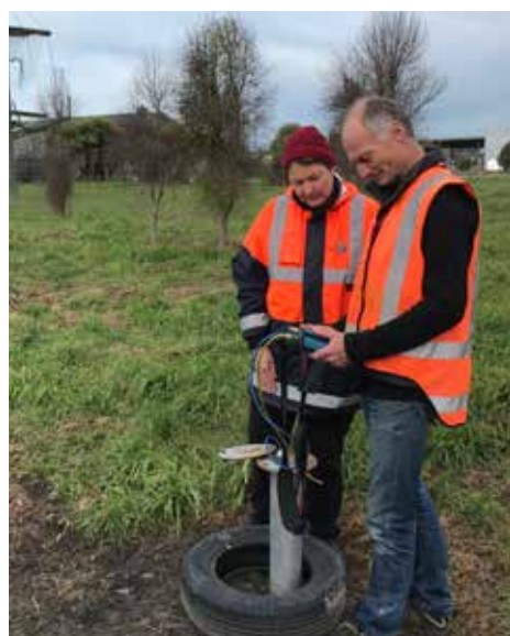
Landfill Gas monitoring
