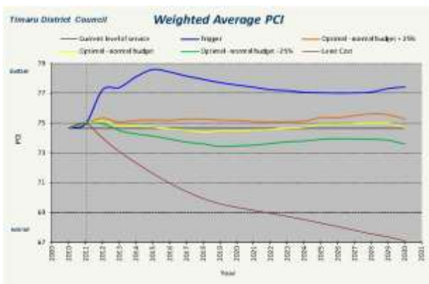
Figure 1: Pavement Condition Index (PCI) - Pavement Base Layers.
