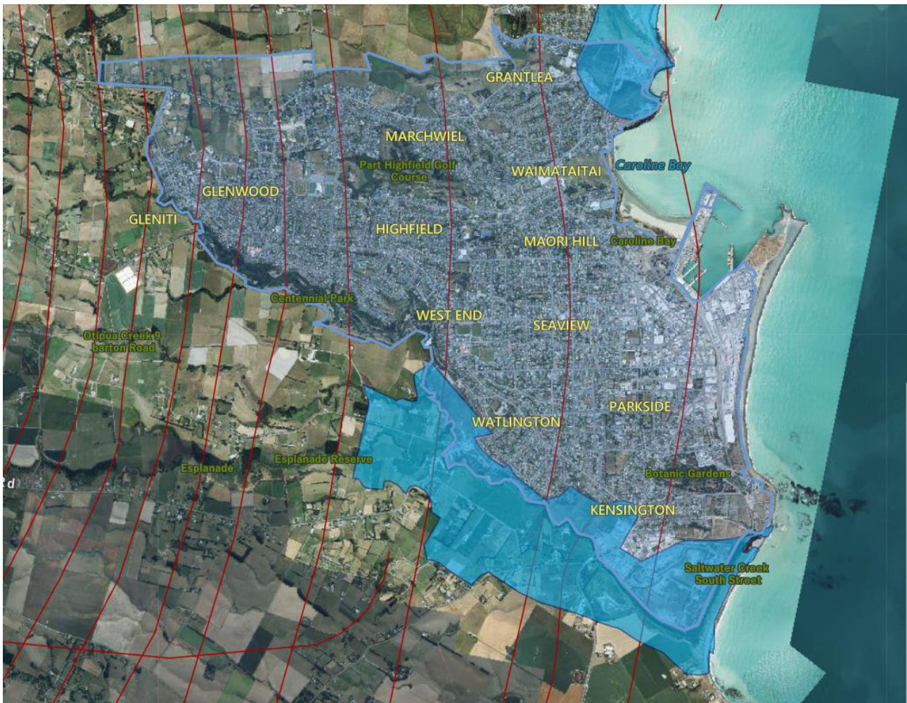
Figure 4-7: Piezometric Contours (red lines) and Semi Confined or Unconfined aquifer (blue shading)
