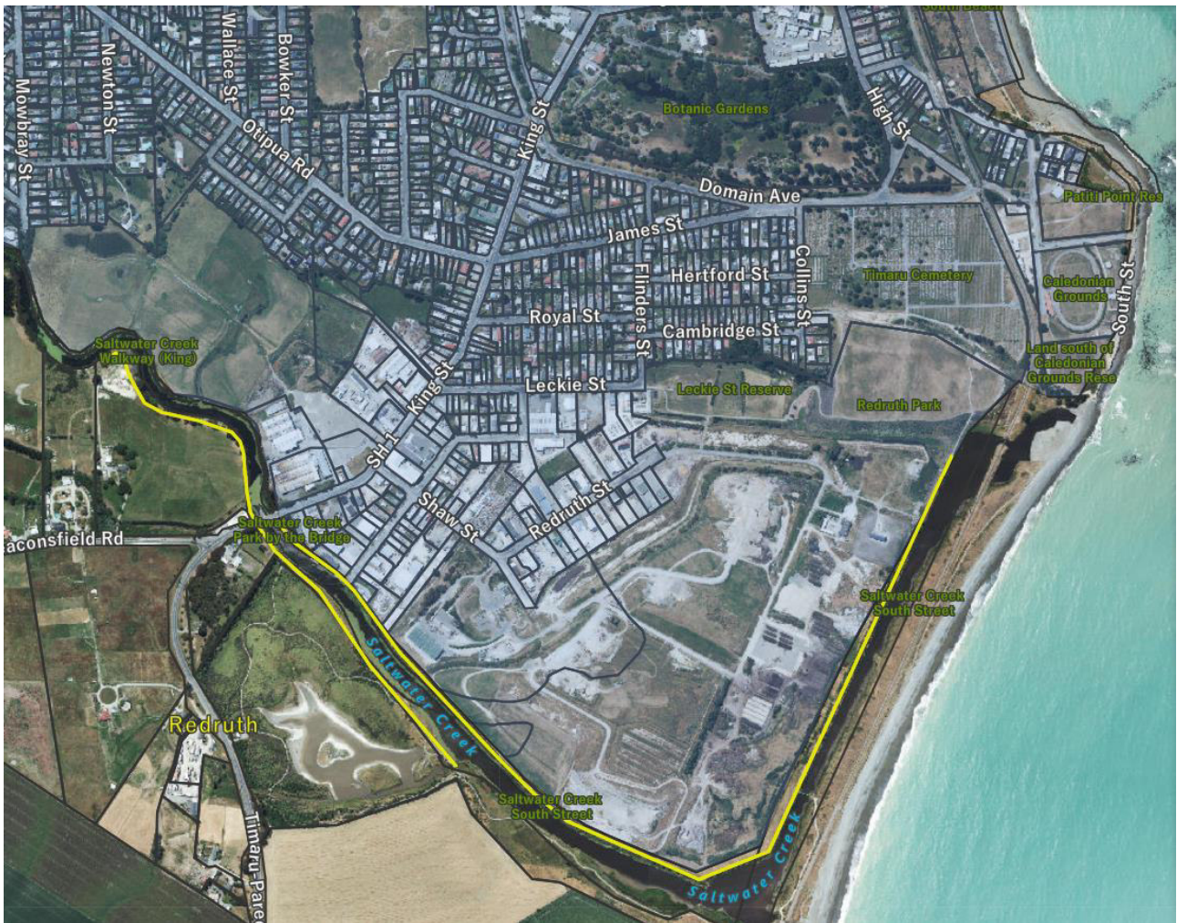
Figure 4-19: Environment Canterbury Stop-bank Infrastructure (yellow lines) at the lower end of Saltwater Creek managed under the Flood Protection Bylaw.
