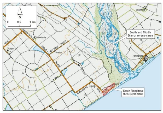
Figure 2-7: Location where South and Middle Branches of the Rangitata River re-enter the main river channel. The natural terrace downstream of this point has historically prevented floodwater continuing down toward the huts
