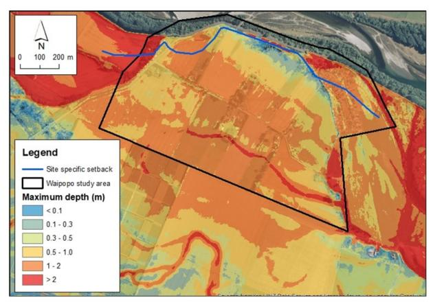
Figure 4-11: Waipopo hut settlement stopbank setback distances and modelled maximum flood depths (elevated scenario with all breakouts occurring)
