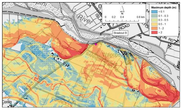
Figure A1-10: Maximum water depth for SH1 breakout flow (700 m³/s) + Breakout B flow (325 m³/s) - elevated scenario
