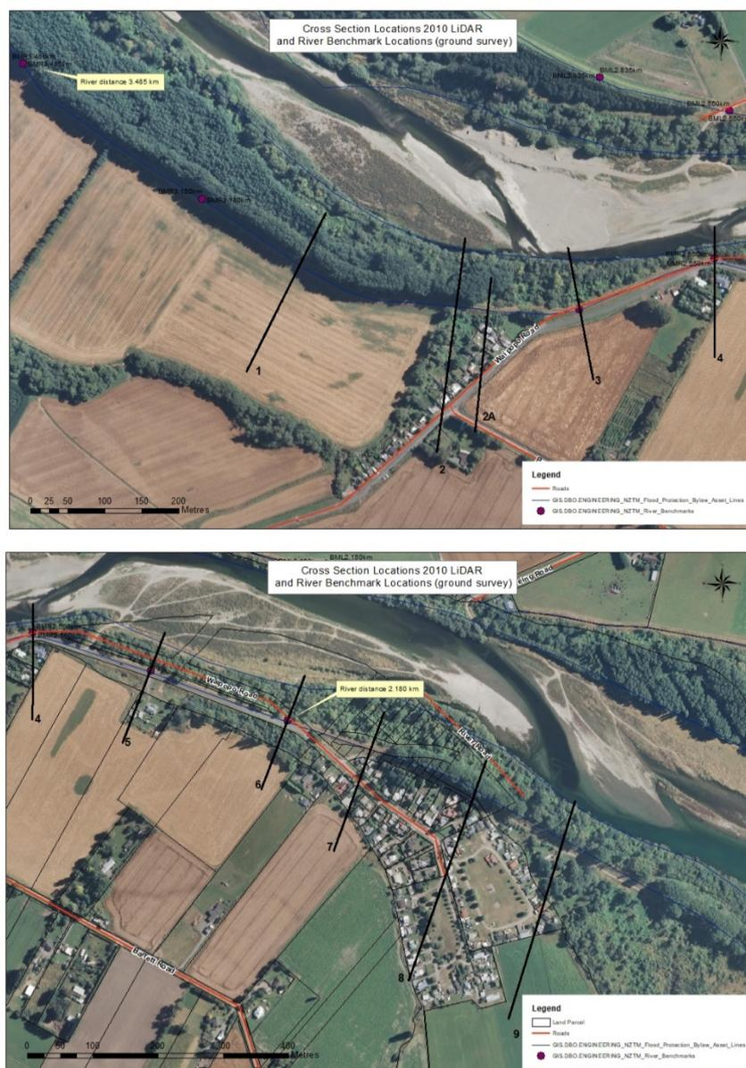
Figure A3-1: Location of cross sections generated to from the 2010 LiDAR as well as river benchmark locations
