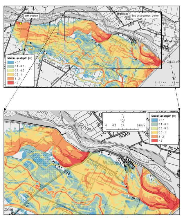
Figure A1-6: Maximum water depth for SH1 breakout flow of 700 m<sup>3</sup>/s - elevated scenario
