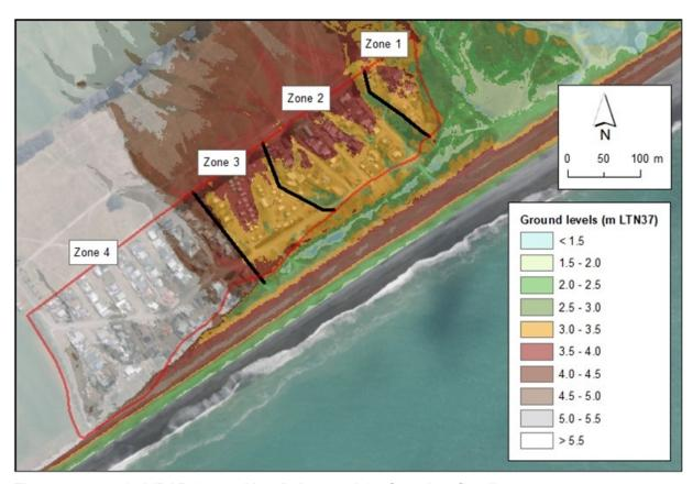
Figure 2-9: 2010 LiDAR (ground level) data, and the four river flooding zones
