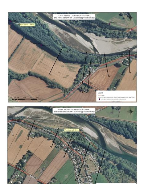
Figure A3-1: Location of cross sections generated to from the 2010 LiDAR as well as river benchmark locations
