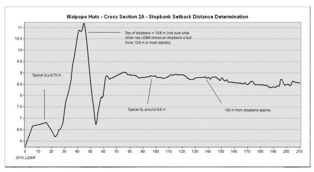
Figure A3-4: LiDAR cross section 2A Waipopo Huts Setback Distance Determination. LiDAR Cross Section 3
