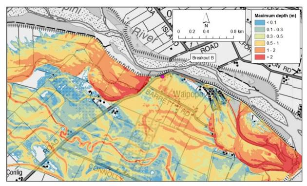
Figure A1-9: Maximum water depth for SH1 breakout flow (540 m³/s) + Breakout B flow (250 m³/s) - base scenario
