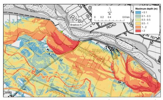
Figure A1-8: Maximum water depth for SH1 breakout flow (700 m³/s) + Breakout A flow (390 m³/s) - elevated scenario
