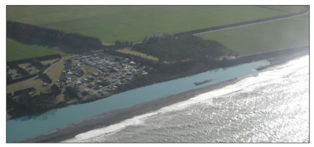
Figure 2-6: Rangitata River mouth on 26 June 2012. Mouth has migrated to north of the north bank huts which are visible in photograph. This was a few days after two huts were inundated at the South Rangitata hut settlement as a result of backwater flooding
