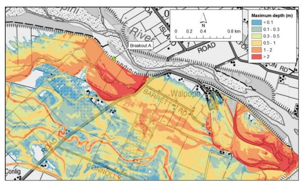
Figure A1-7: Maximum water depth for SH1 breakout flow (540 m³/s) + Breakout A flow (300 m³/s) - base scenario
