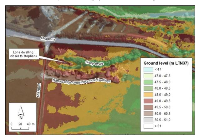
Figure 6-3: 2010 LiDAR (ground level) data for the Mill Road hut settlement area
