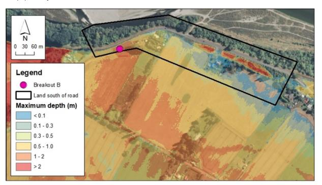
Figure 4-18: Modelled maximum flood depths for elevated SH1 and B breakouts south of road
