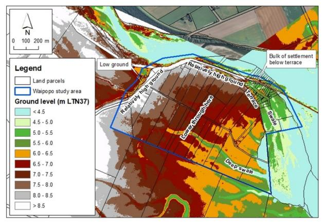
Figure 4-5: 2010 LiDAR (ground level) data for the Waipopo hut settlement area
