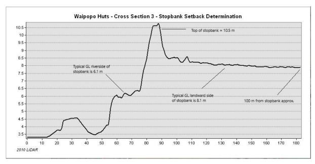
Figure A3-5: LiDAR cross section 3 Waipopo Huts Setback Distance Determination. LiDAR Cross Section 4
