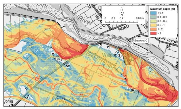
Figure A1-11: Maximum water depth for SH1 breakout flow (540 m³/s) + Breakout C flow (320 m³/s) - base scenario
