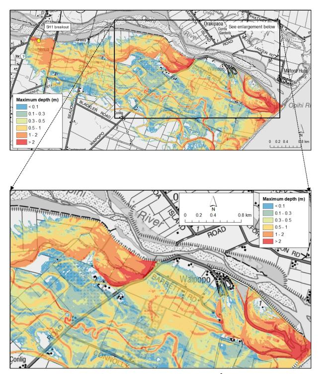
Figure A1-5: Maximum water depth for SH1 breakout flow of 540 m³/s - base scenario
