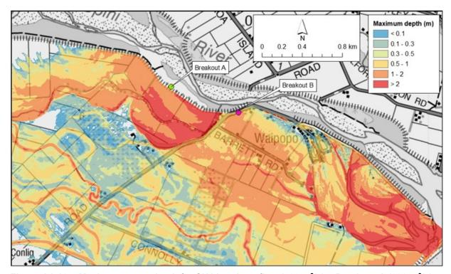
Figure A1-13: Maximum water depth for SH1 breakout flow (700 m³/s) + Breakout A (390 m³/s) + Breakout B (325 m³/s) - elevated scenario
