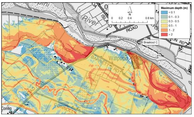
Figure A1-12: Maximum water depth for SH1 breakout flow (700 m³/s) + Breakout C flow (415 m³/s) - elevated scenario
