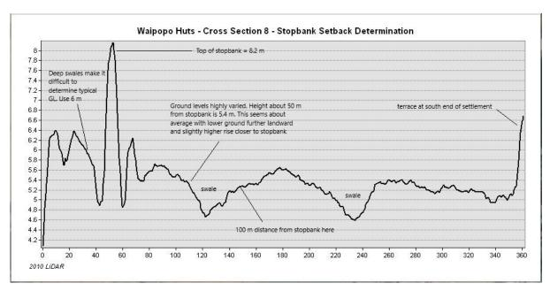
Figure A3-9: LiDAR cross section 8 Waipopo Huts Setback Distance Determination, LiDAR Cross Section 9
