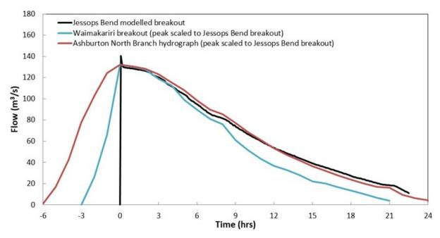
Figure A1-4: Comparison of breakout flows and Ashburton North Branch flood hydrograph (scaled to match Jessops Bend peak breakout flows)
