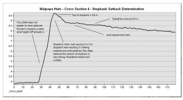
Figure A3-6: LiDAR cross section 4 Waipopo Huts Setback Distance Determination, LiDAR Cross Sections 5 & 6
