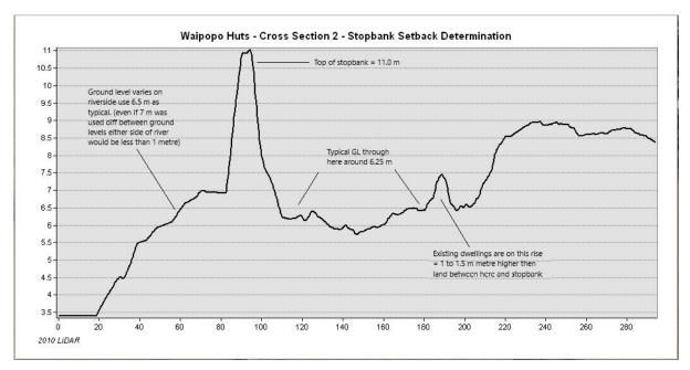
Figure A3-3: LiDAR cross section 2 Waipopo Huts Setback Distance Determination LiDAR Cross Section 2A
