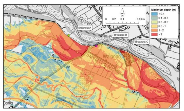
Figure A1-14: Maximum water depth for SH1 breakout flow (700 m³/s) + Breakout A (390 m³/s) + Breakout B (325 m³/s) + Breakout C (415 m³/s) - elevated scenario
